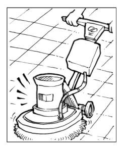
Floor scrubbing machines should be discharged to a sanitary sewer – never to a storm drain or swale.
