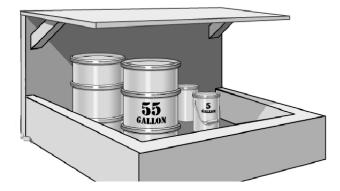
Figure A2-1 Example of Outdoor Storage with Roof and Secondary Containment
